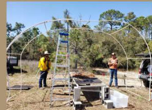
Stable frame to support our rain simulator positioned above our slope burn table and sample collection system.
