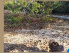
Extraction site for sample soil. Topsoil was manually removed to decrease the amount of organic matter from the sample.
