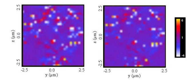
Left: Dislocation density tensor component  $\alpha_{12}$  (mrad/µm)
