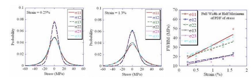
• Pair correlation of internal stress fields of dislocations in deformed Cu
