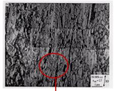
A volume of deformed crystal showing mesoscale deformation features
