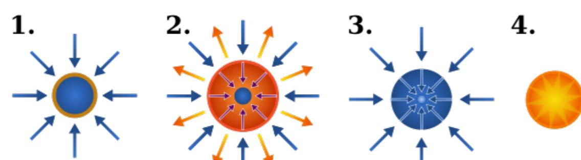
Figure 1: (The ICF Process) 1) Lasers heat the surface of the target. 2) Surface material is ablated causing the fuel core to implode. 3) Final stage of fuel implosion, very high density fuel ignites. 4) Thermonuclear burn front propagates outward through compressed fuel causing ignition and producing much more energy than what was needed to initiate the process.
