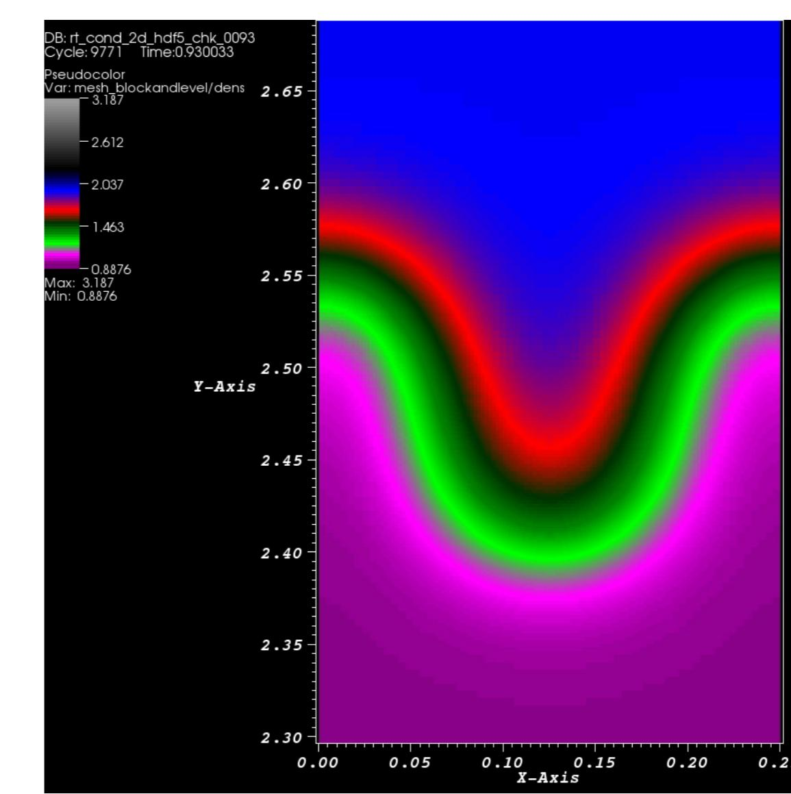
Figure 3: RTI with Constant Thermal Conduction in Nonlinear Regime - The Density Field.
