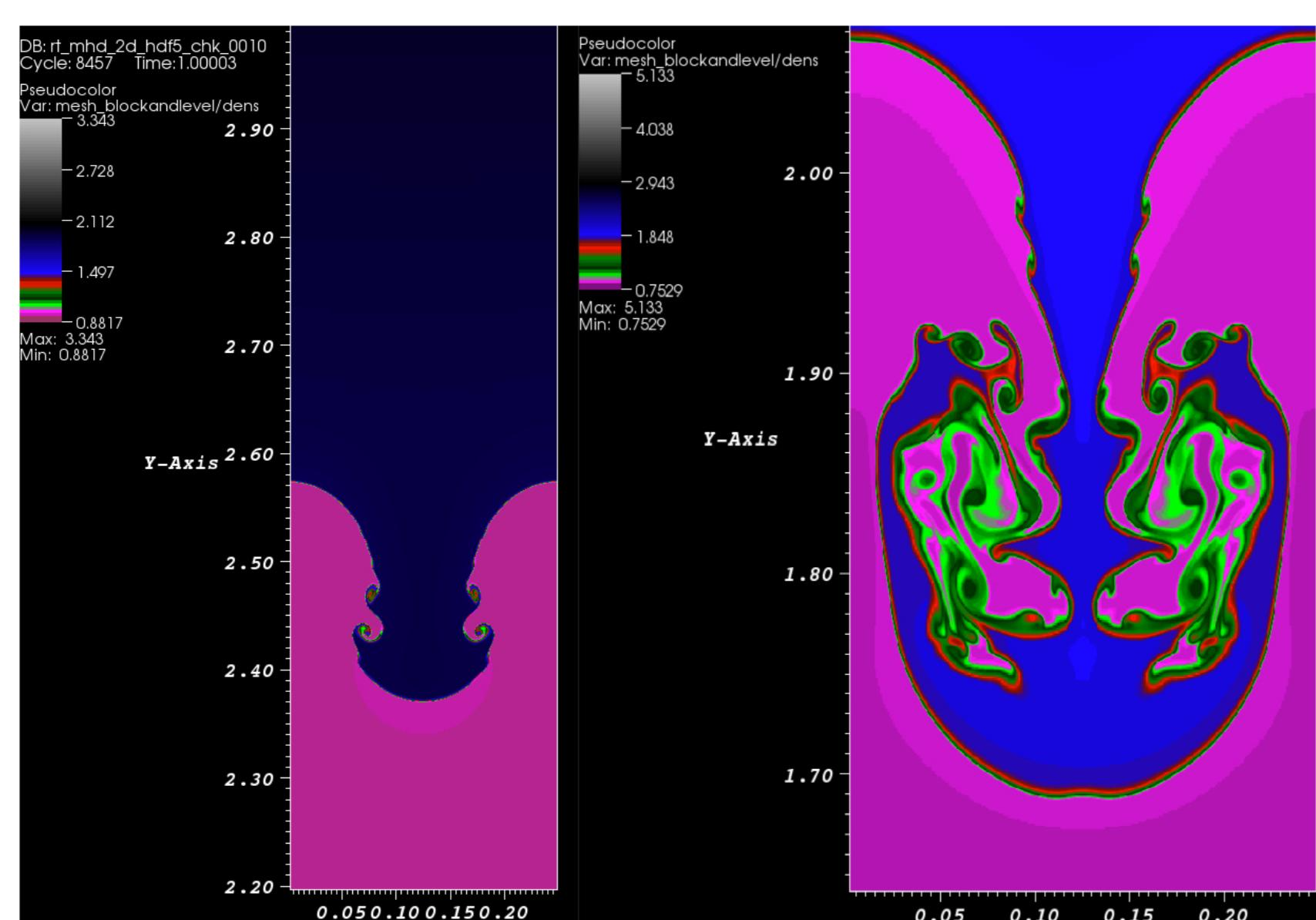
Figure 2: RTI in the Linear and Nonlinear Regime - The Density Field.
