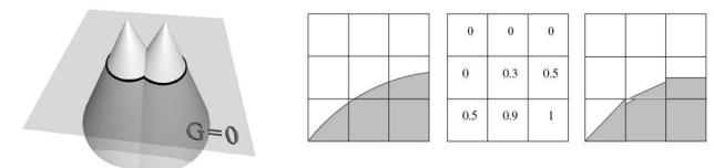
Figure 7 : (left panel) Illustration of a signed distance function representing the interface being tracked using the level set method. [8] (right panel) Illustration of volume fractions and interface reconstruction using the volume of fluid method. [9]
