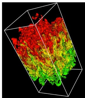
Figure 1 : A rendering of density from a validation simulation of the Rayleigh-Taylor instability. [1]
