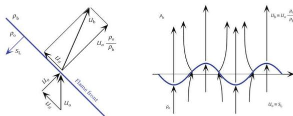
Figure 5 : (left panel) The split of the flow velocity into tangential and normal components is shown. Notice that the tangential component remains fixed, but the normal component jumps. (right panel) The LD mechanism in the context of a wrinkled flame. [6]
