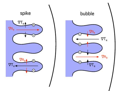
Figure 6 : The Biermann battery mechanism at the RT-unstable interface. The magnetic field is generated at the interface due to misalignment of gradients of electron number density and electron temperature. A similar situation arises at the wrinkled flame front [7]
