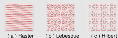
Figure 5: Examples of space-filling curves in two dimensions (order=4)
