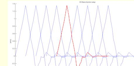
Figure 4. Scaling basis function D6, and the translates where the derivative inner products are non-zero
