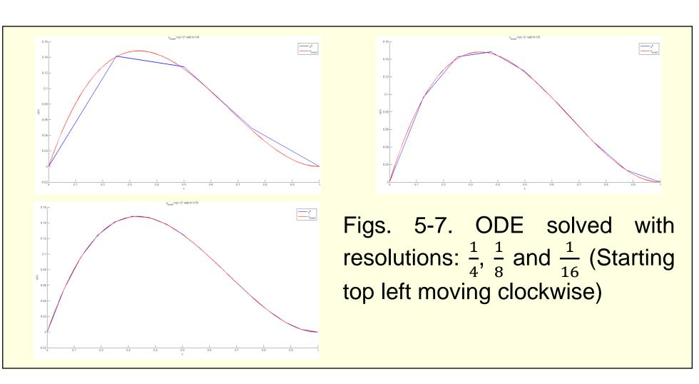
From the plots in figures 5-7 we see that the Wavelet-Galerkin method appears to approach the actual solution as we hoped. Using the exact solution and the computed solutions at a number of discretization's we can calculate the rates of convergence as the resolution is increased. Remember that h is calculated with respect to  $2^m$  so as we increase m, the resolution is also increased
