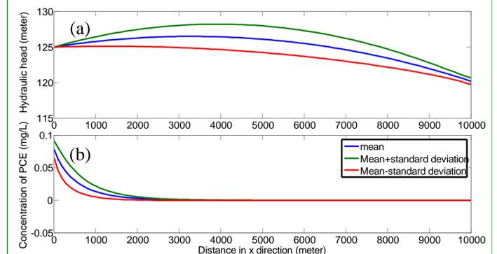
Figure 6. The mean and standard deviation of hydraulic head (a) and PCE concentration (b) plotted simultaneously for the whole domain.
