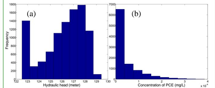
Figure 5. Hydraulic head (a) and concentration of PCE (b) distributions at location  $x = 5000$  meters.
