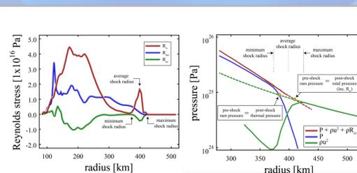
Figure 6: (left panel) Reynolds stress components for the same nominal model as in Fig. 5 (at 100ms). (right panel) Investigation of the contributions from the radial Reynolds stress to the nominal shock position, as proposed by Murphy et al. [5]. Note that the correction utilizing  $R_{rr}$  still lies within the maximum extent of the shock, casting doubt on the importance Reynolds stresses in these models.
