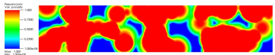
This field has an average porosity of 0.7729 and an average permeability from (2) of  $1.432 \times 10^{-4} \text{ mm}^2$ . It can be compared to an SEM image of a foam that was held under a low temperature mold:
