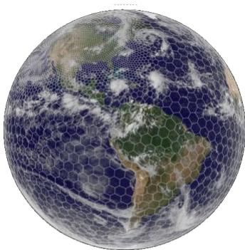
Figure 1: A highly nonuniform mesh of the Earth that resolves climatic phenomena at multiple scales. Although this mesh provides multi-resolution abilities in simulations, the smallest sized cells limit the time step of the simulation, requiring new time integration techniques to enhance simulation performance.
