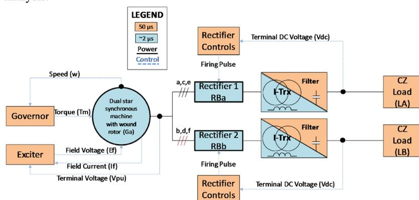
Figure 1: PGM model under investigation. The different colored components are simulated by different time steps.
