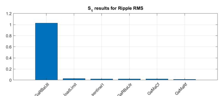
Figure 4: Final results of the first order sensitivity indices for all the considered variables. The filter inductance has a dominant influence on the voltage ripple RMS value. There is some intrinsic randomness in the approximated values. This is why the index for sentinel1 (the non-influential variable) is not zero as it should be. However, the stochastic nature of the analysis should not change the conclusions of the analysis.
