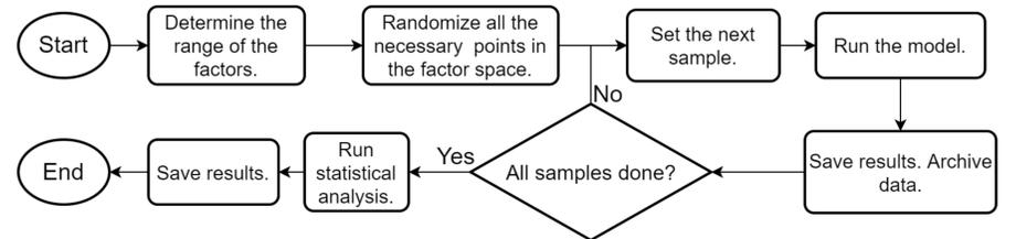
Figure 2: The automated process of gathering the samples for First order sensitivity index calculations.
